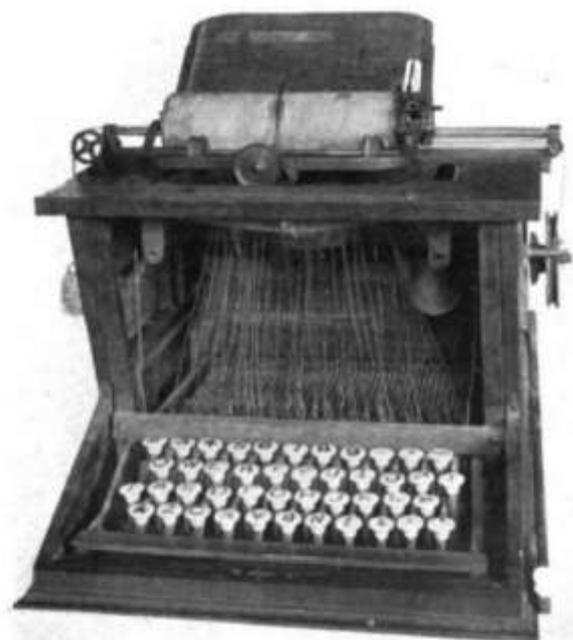
**Prototype of the Sholes and Glidden typewriter, 1873, the first commercially successful typewriter, and the first with a QWERTY keyboard.**
