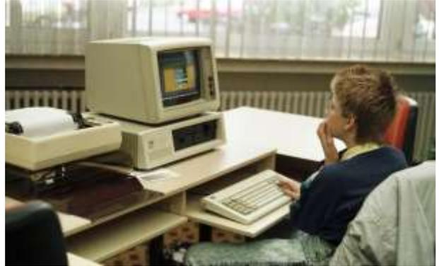
**IBM Computer 1981. Note the elevated position of the monitor but much lower keyboard compared to the 1960's typewriter.**
