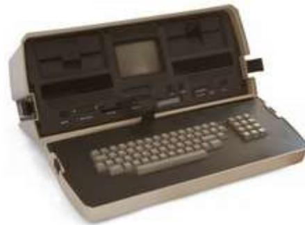
**Osborne I 'portable' computer – 1981 – 10 kgs, no battery and tiny screen.**
